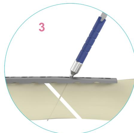
Hexagonal Screwdriver 3,5 mm (A3200-0211) is used to drive the screw. As the screw is driven it pulls the other cortex towards the first cortex and compressin at the fracture site is achieved.
