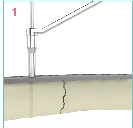
Tap Cancellous 5,0 mm (A3200-0206) is coupled to the T-Handle Quick Coupling (A3200-0223), Neutral And Load Drill Guide (A3200-0214) is turned, 4,5 mm direction of the handpiece is used for tapping both cortex of the screw hole.
